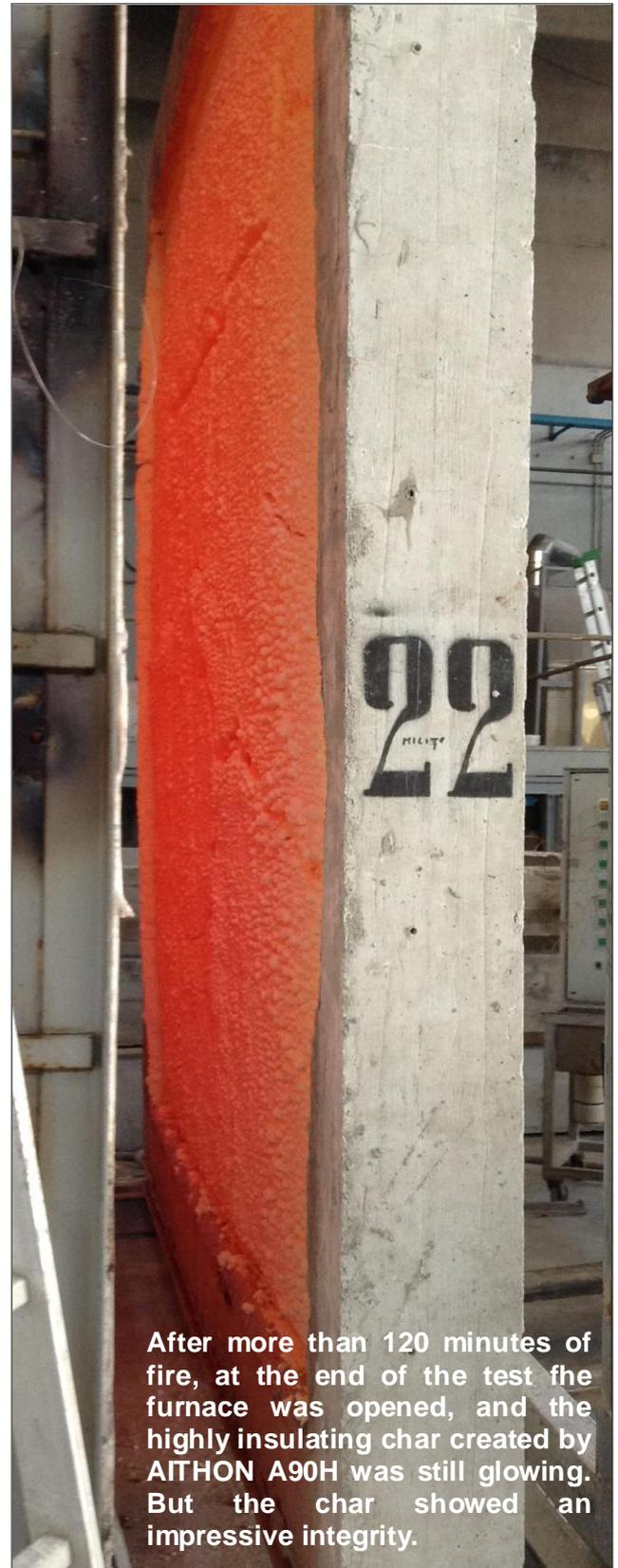
After more than 120 minutes of fire, at the end of the test the furnace was opened, and the highly insulating char created by AITHON A90H was still glowing. But the char showed an impressive integrity.
